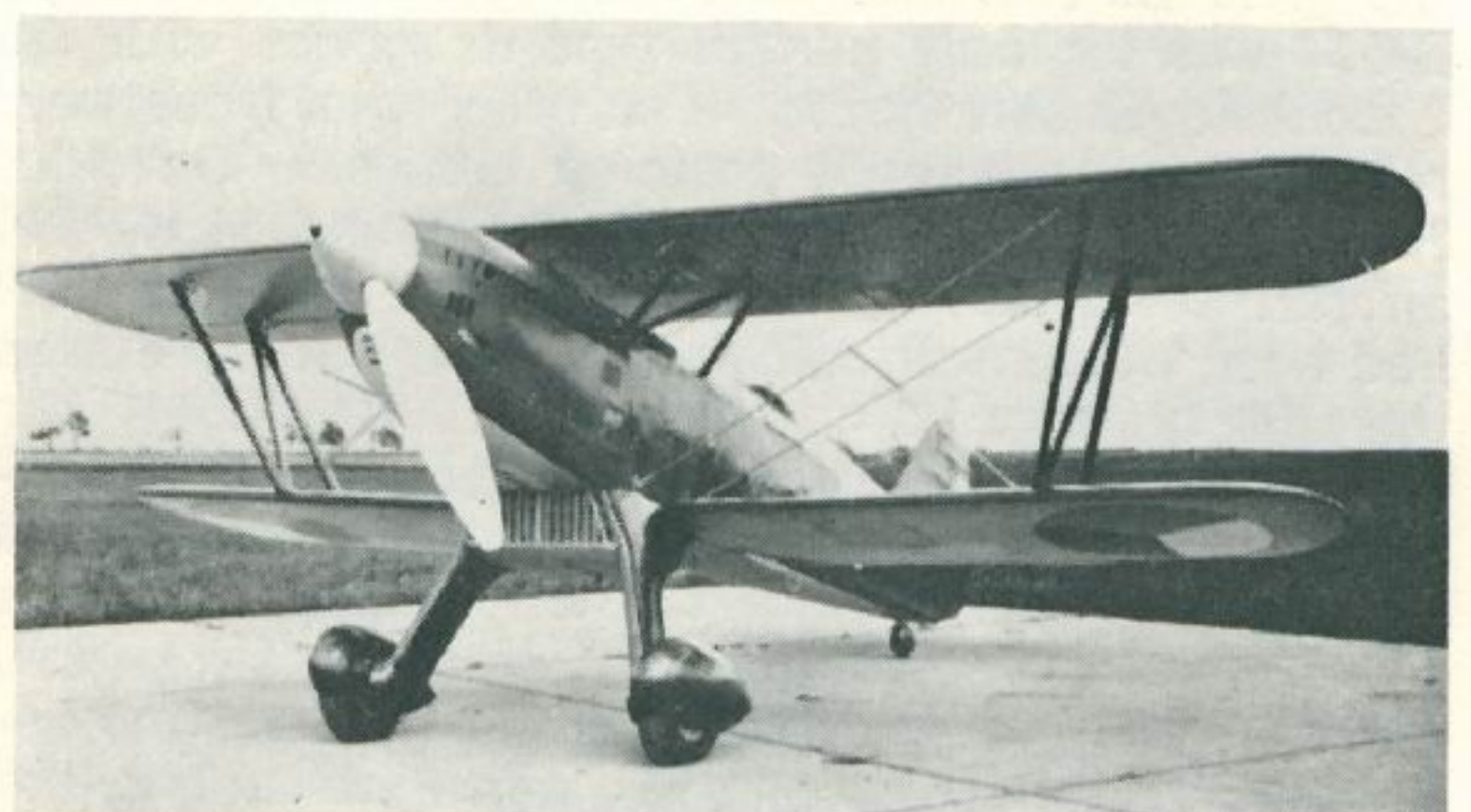
(Top left & right) The Avia B-534 in the first, second, (middle left & right) third and fourth production series configurations; (bottom left) the Bk-534, with a third 7.7 mm. gun between the cylinder banks; and (right) the B-634 of 1936 with cantilever undercarriage. (Photos: Avia)
